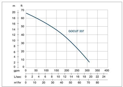
Shaft Speed: 2850 rpm Outlet: 80mm, 3in **OUTPUT HEAD FLOW**
